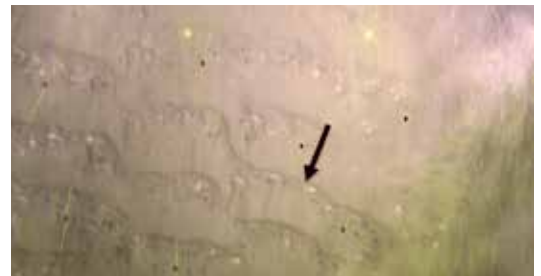
A still image from a video of the seafloor. The black arrow shows the direction of the tide, the yellow stripes are measurements used to determine the length of sand ripples.
